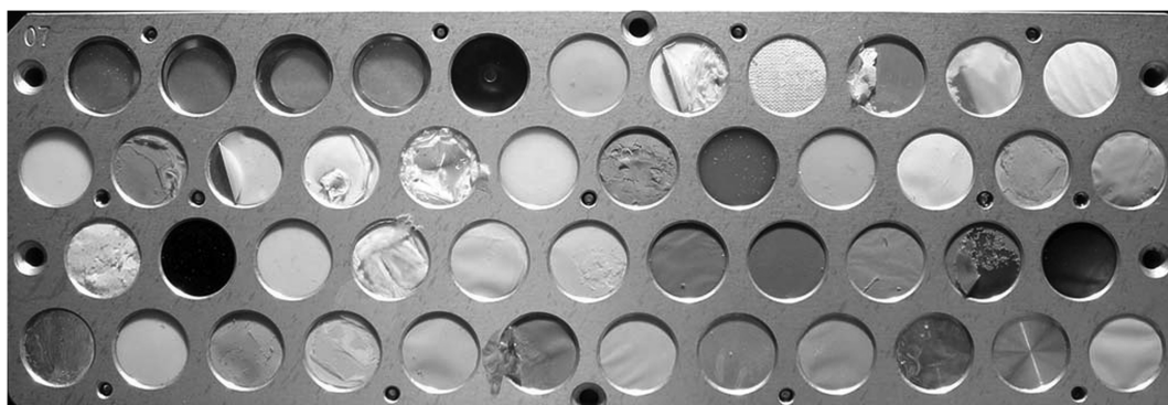
Fig. 3 Photograph of the MISSE 2 PEACE polymers experiment postflight.
