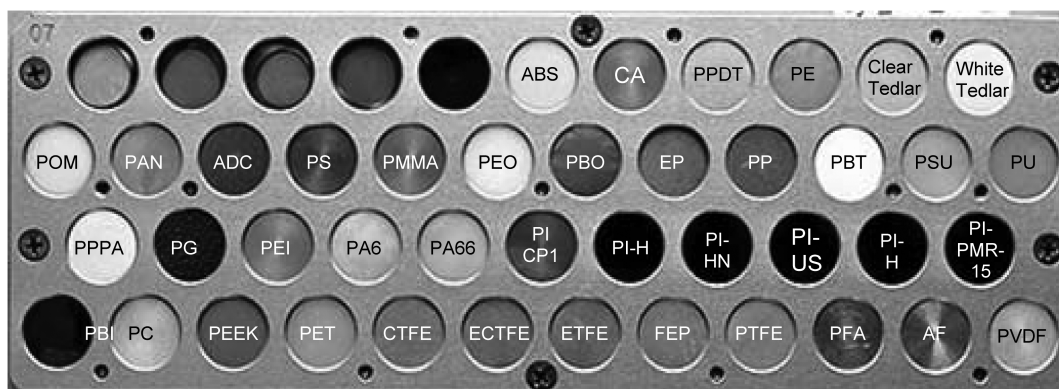
Fig. 2 Photograph of the MISSE 2 PEACE polymers experiment before flight. The labels shown indicate the materials defined in Table 1.
